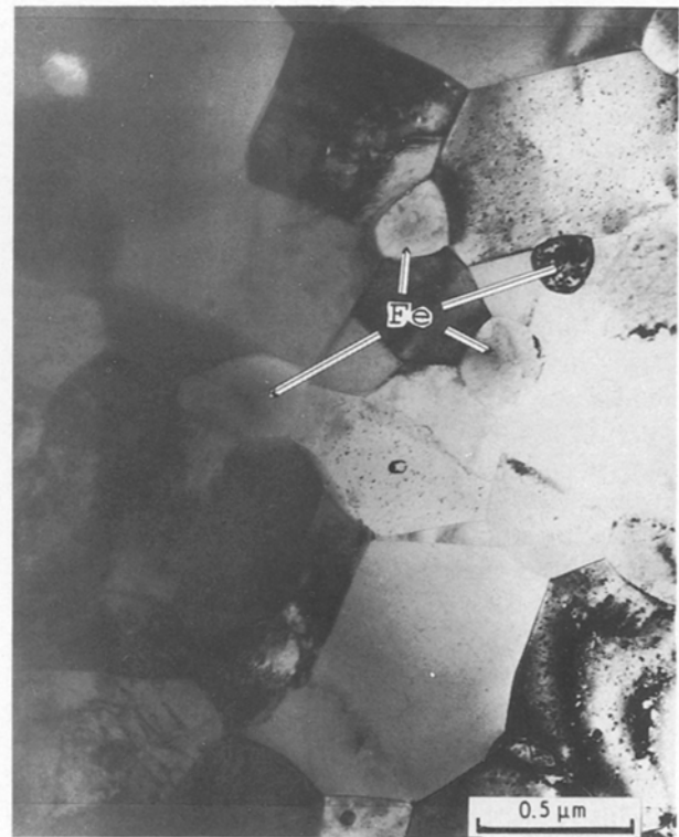
Figure 9 TEM micrograph of transverse section of Cu-20%Fe drawn to \eta = 8.1 and annealed for 24 h at 600 °C
