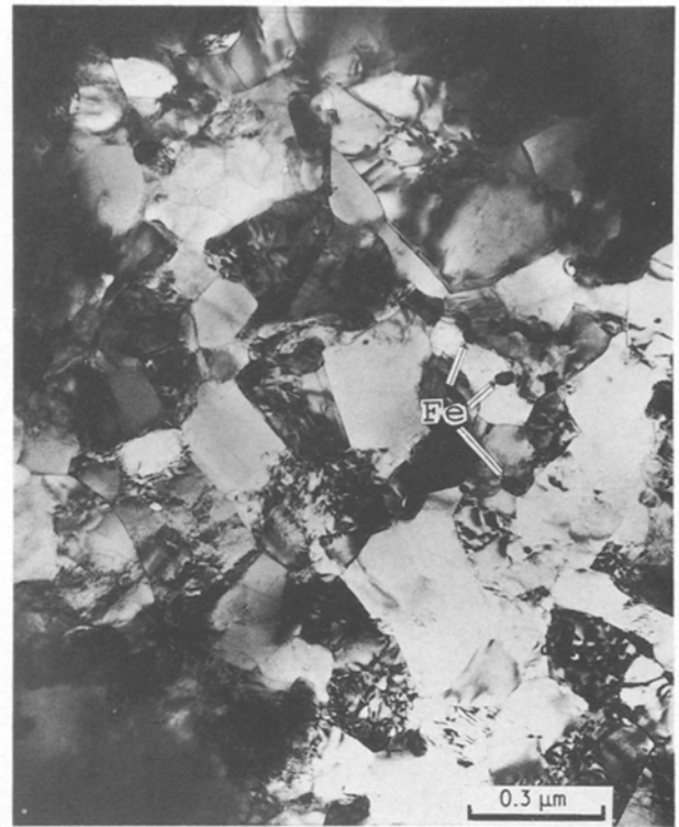
Figure 8 TEM micrograph of transverse section of Cu-20%Fe drawn to \eta = 8.1 and annealed for 24 h at 300 °C.
